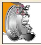
Advanced 'Shift Plane' software reduces the weight and time required to balance. With 1 push of a button, you can shift the corrective weight position on the wheel to see the effect on the weight required, potentially saving weights and re-spin time.
