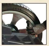
Model M-3200 offers the ability for the technician to program in whether they prefer to apply weights at 3:00, 6:00 or 12:00 on the wheel. Balancer automatically recalculates amount dependent on what is easier for the technician.
