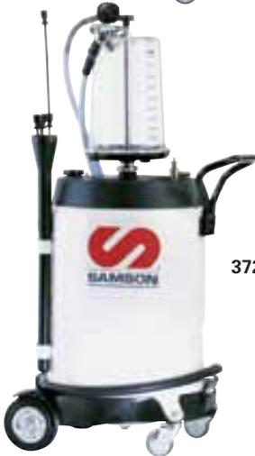
Discharge is carried out through a 6.5 foot discharge hose pressurizing the unit at 7 psi using a tire inflator.
